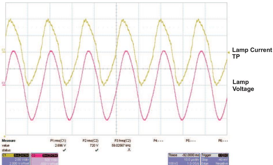
Figure 2. Lamp 1 VSEN Test Point and Lamp 1 Voltage
