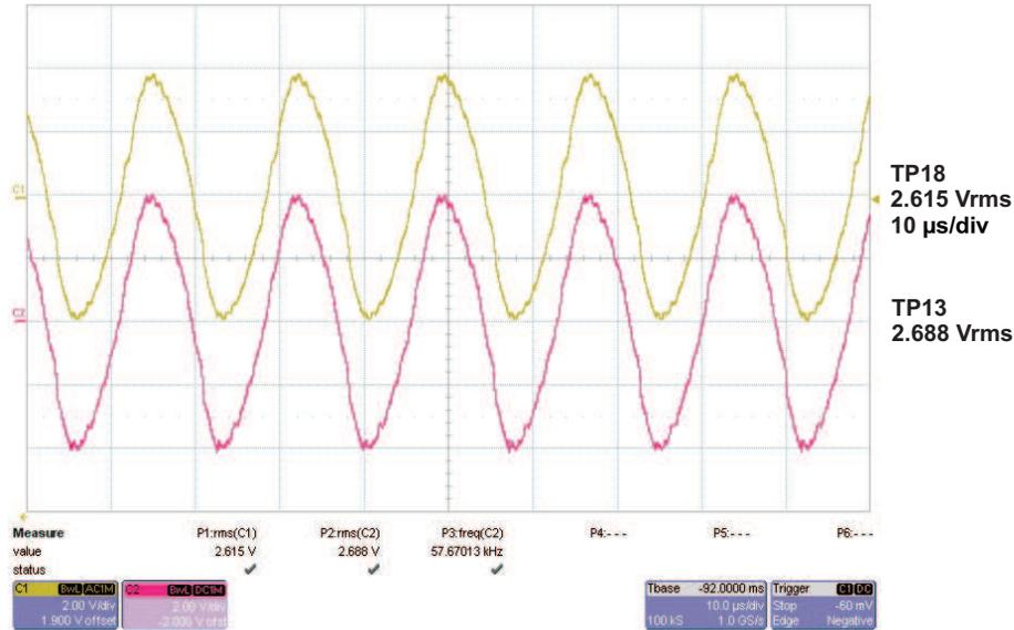
Figure 3. Lamp 1 and Lamp 2 CSEN Test Point
