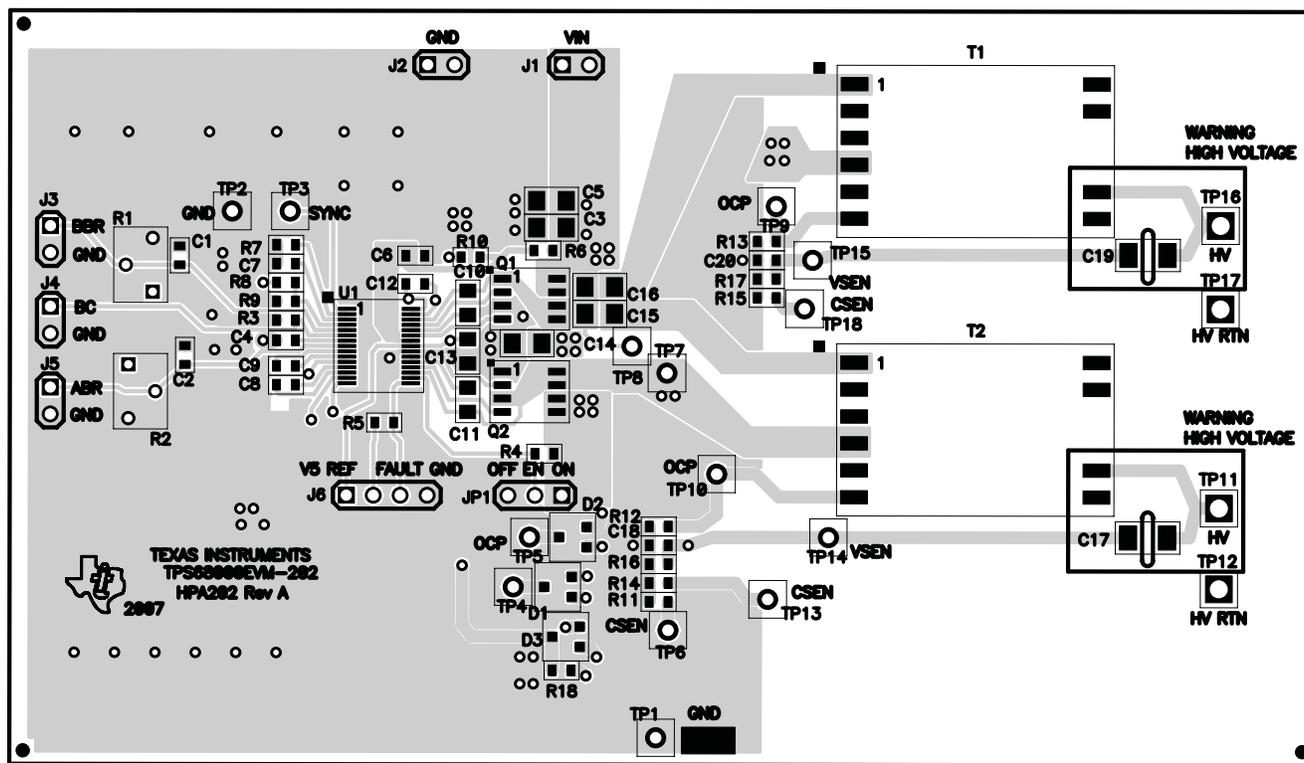
Figure 9. Assembly Layer
