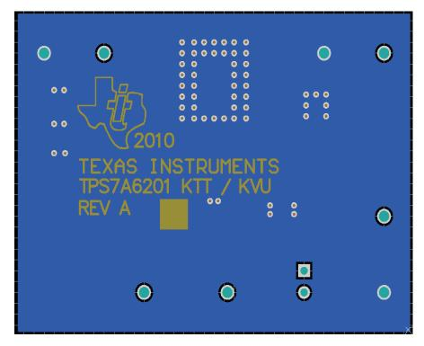
Figure 4. Bottom Assembly Layer
