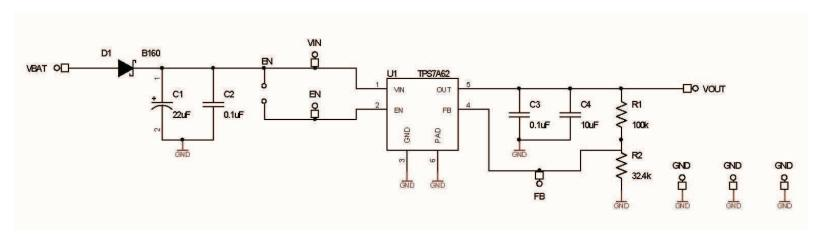
Figure 5. TPS7A6201QKTT EVM Schematic
