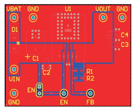
Figure 2. Top Assembly Layer
