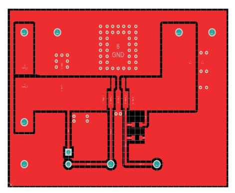
Figure 3. Top Layer Routing
