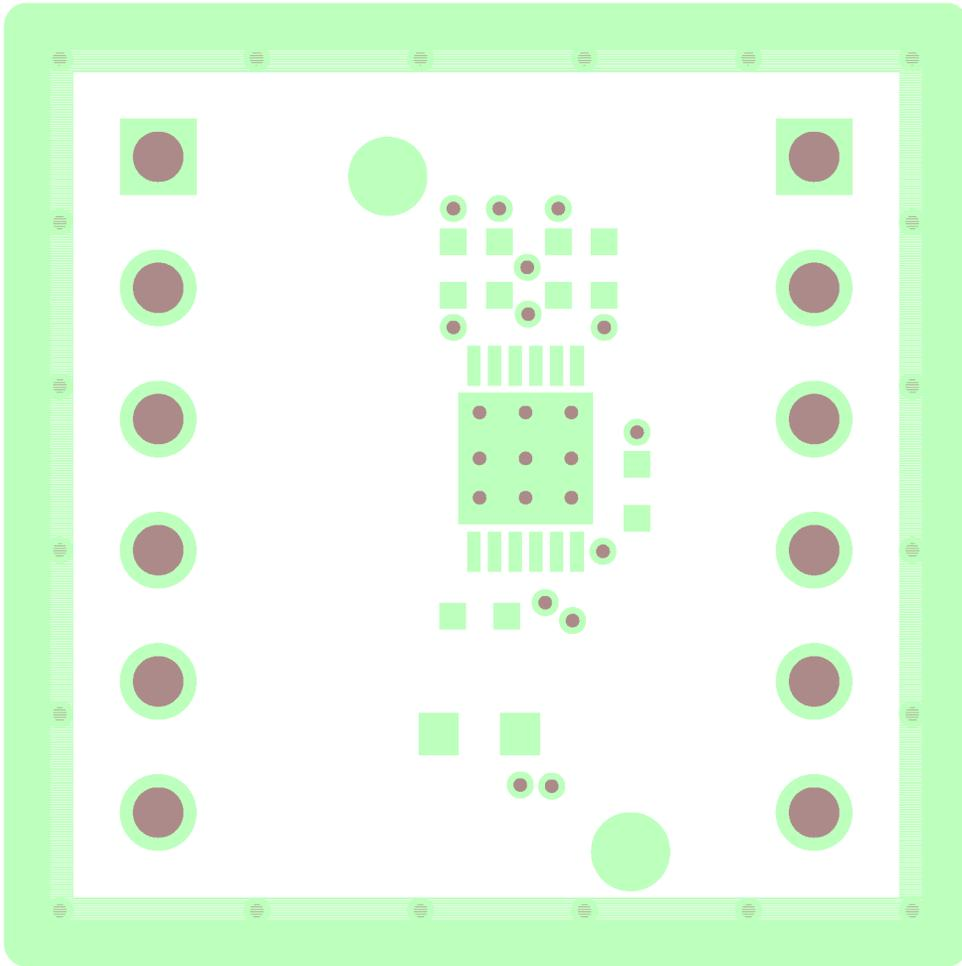
**Figure 5. SMP-BQ27410G1-MVK Board Solder Mask – Top Side**
