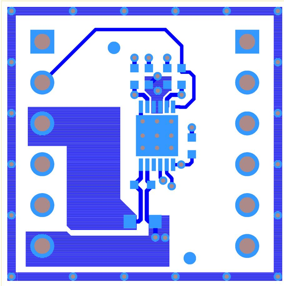
**Figure 6. SMP-BQ27410G1-MVK Board Layer 1 – Top Side**
