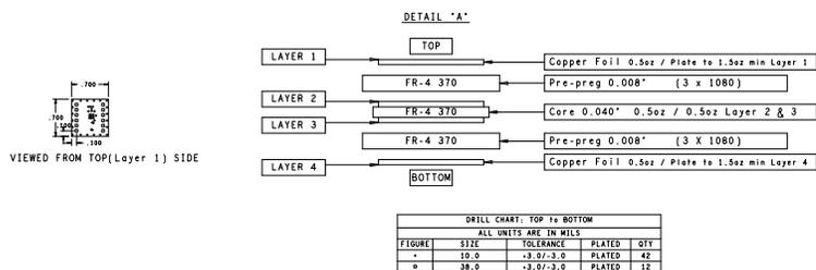
Figure 13. SMP-BQ27410G1-MVK Fabrication Drawing
