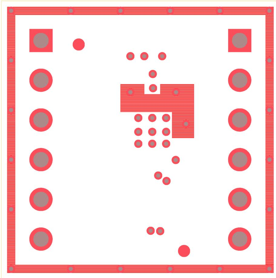
**Figure 9. SMP-BQ27410G1-MVK Board Layer 4 – Bottom Side**
