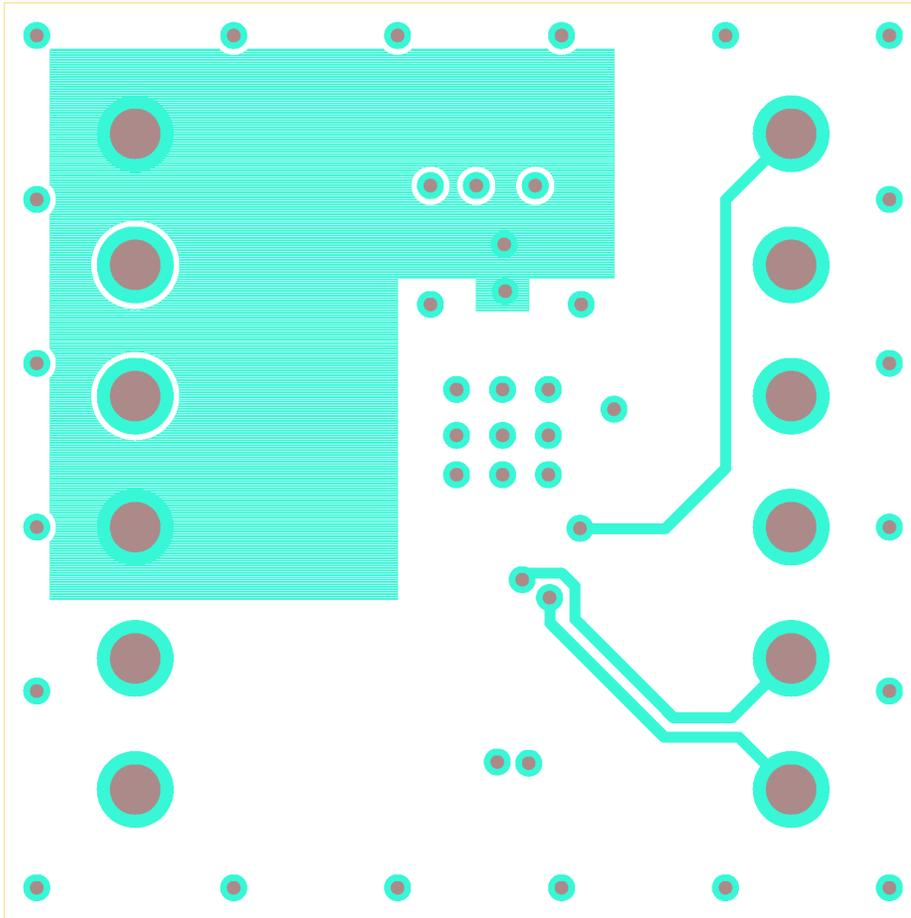
**Figure 8. SMP-BQ27410G1-MVK Board Layer 3 – Signal**
