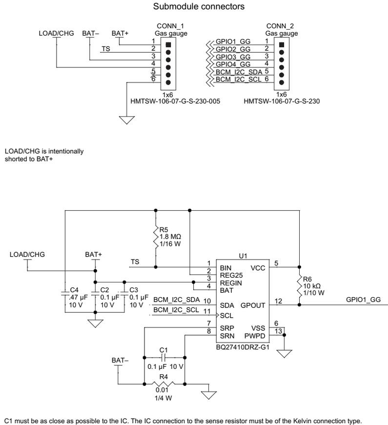
Figure 12. SMP-BQ27410G1-MVK Schematic
