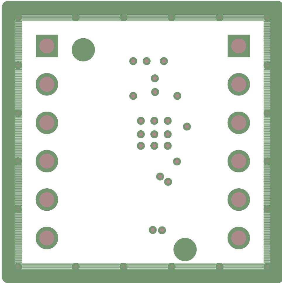
Figure 10. SMP-BQ27410G1-MVK Board Solder Mask – Bottom Side
