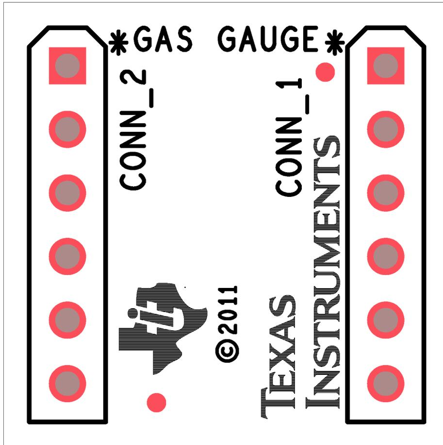
Figure 11. SMP-BQ27410G1-MVK Board Silkscreen – Bottom Side
