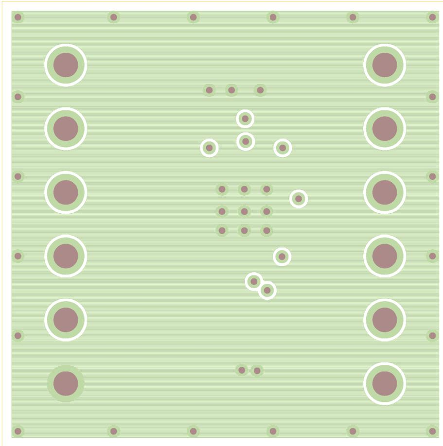
**Figure 7. SMP-BQ27410G1-MVK Board Layer 2 – Ground Plane**
