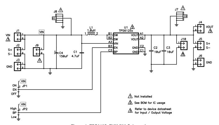
Figure 1. TPS6125xEVM-766 Schematic
