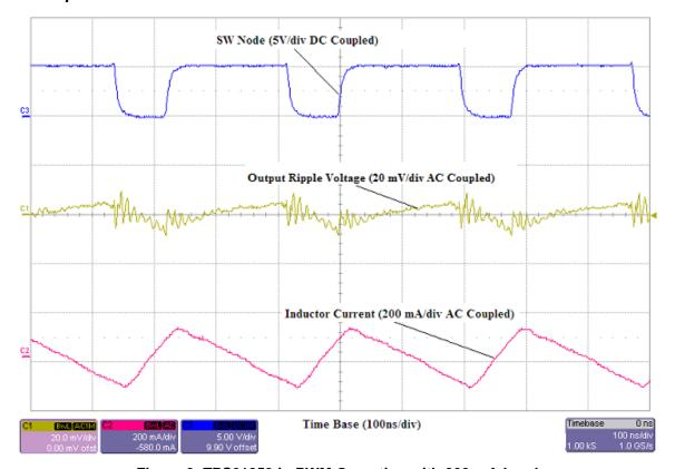
Figure 3. TPS61253 in PWM Operation with 260-mA Load
