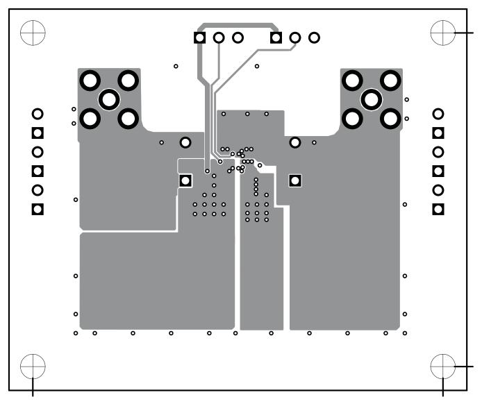
Figure 10. TPS6125xEVM-766 Bottom Copper (Viewed from Bottom)
