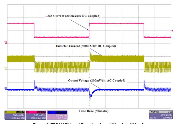
Figure 4. TPS61253 Load Transient from 100 mA to 300 mA
