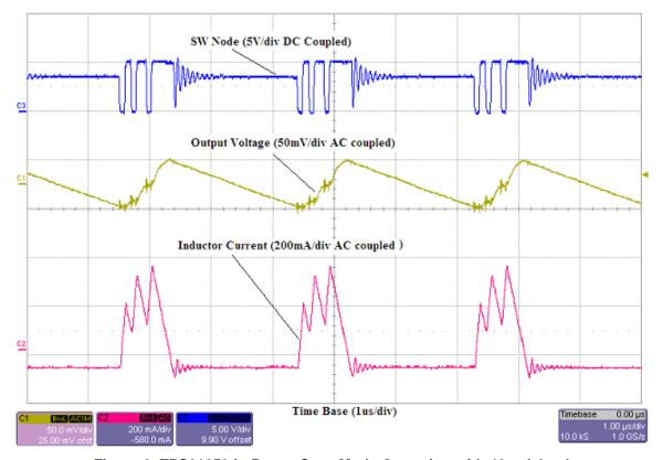
Figure 2. TPS61253 in Power Save Mode Operation with 40-mA load
