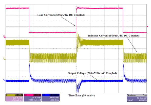
Figure 5. TPS61253 Load Transient from 100 mA to 500 mA
