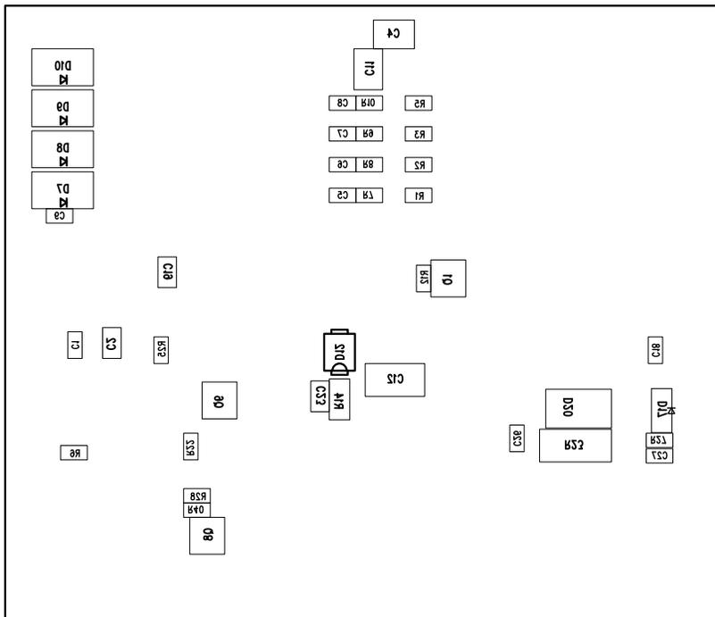
Figure 12. Bottom-Side Placement
