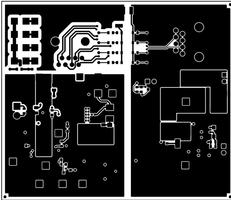
Figure 11. Bottom-Side Routing
