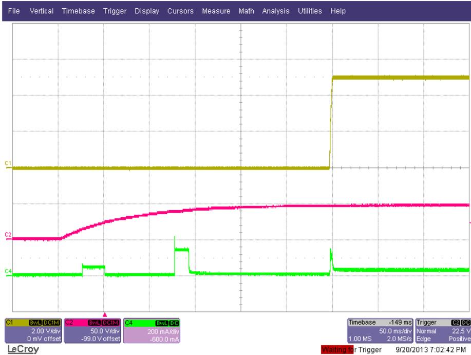
The scope plot below shows the 5V output voltage startup waveform after the application of 48Vdc at J1 (Ethernet connector. The output was loaded to 4.5A using an electronic load in CR mode.
