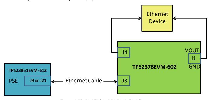
Figure 4. Typical TPS2378EVM-602 Test Setup
