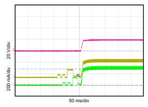
Figure 5. Startup Response to 26-W Load for a 48-V Input
