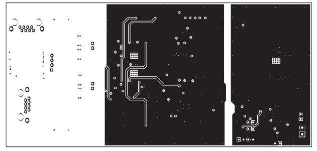
Figure 11. Layer 3 Routing
