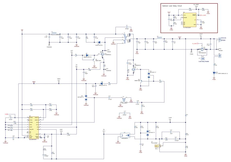
Figure 3. TPS2378EVM-602 DCDC Converter Section
