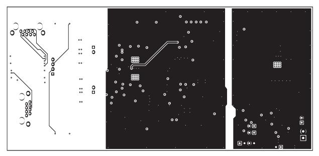
Figure 10. Layer 2 Routing
