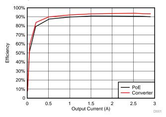
Figure 7. Efficiency of the TPS2378EVM-602
