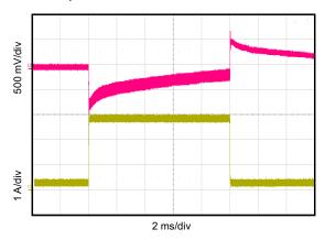
Figure 6. Transient Response from 290 mA to 2.9 A for a 48-V Input
