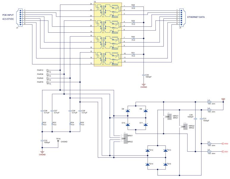
Figure 1. TPS2378EVM-602 PD Front-End Schematic
