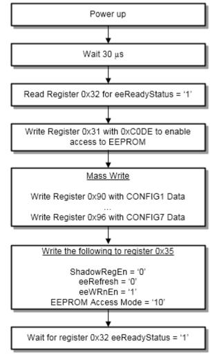
Figure 8. DRV10983-Q1 and DRV10987 Mass Write Protocol Using I<sup>2</sup>C
