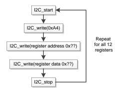
Figure 1. I<sup>2</sup>C Command Chain for Enabling Sidata Bit
