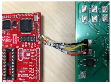
Figure 62. LaunchPad<sup>™</sup> Connected to TIDA-01373
