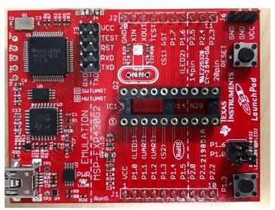
Figure 61. LaunchPad<sup>™</sup> MSP430<sup>™</sup> Socket (Depopulated)
