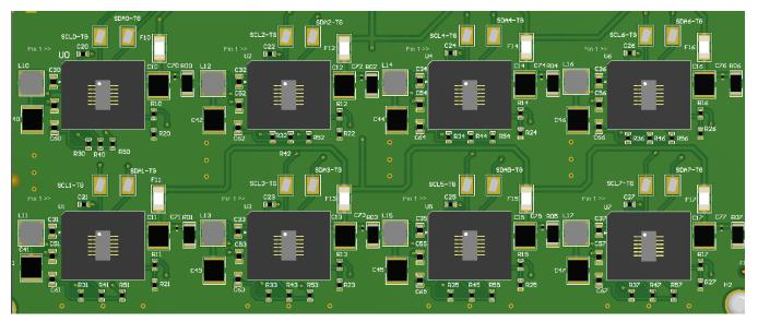
Figure 24. Sockets With Device Populated in Proper Orientation
