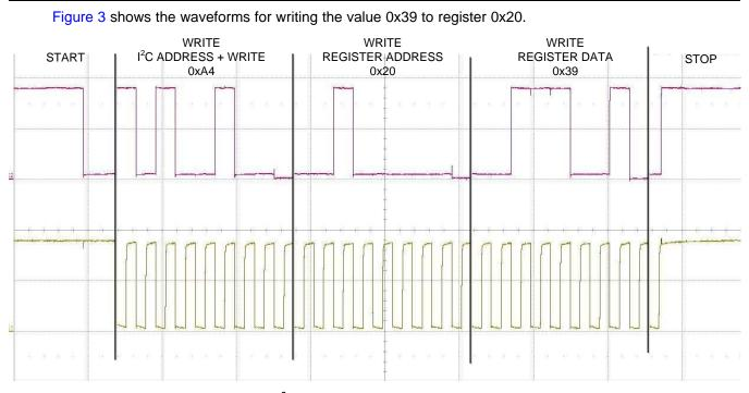
Using <sup>P</sup>C to Communicate With the DRV10983 and DRV10975 Motor Drivers
