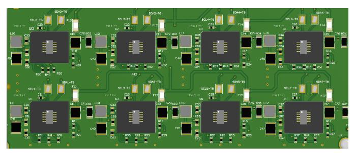
Figure 48. Sockets With Device Populated in Proper Orientation
