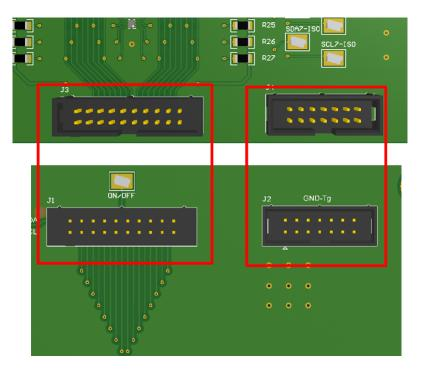
Figure 23. Ribbon Wire Headers on Both Boards
