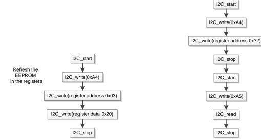
Figure 5. I<sup>2</sup>C Command Chain for Refreshing the Registers
