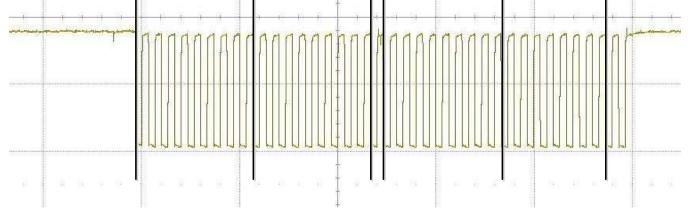
Figure 7. I<sup>2</sup>C Waveform of Reading a Register
