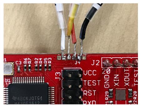
Figure 60. LaunchPad<sup>™</sup> 4-Pin Programming Header with Soldered Wires
