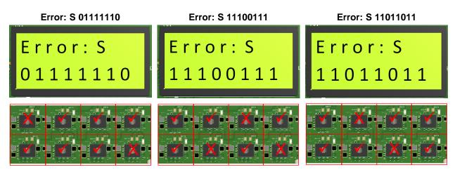
If 8 devices have been placed in the socket and the system still gives this error message, it means that one of the devices was incorrectly placed in the socket; either the leads are not all properly touching or it was place in upside-down. If you wish to replace the IC in the socket then power down the TIDA-01373 with the ON/OFF switch by switching it to 'OFF' and start back at Section 5.3.2.1.
