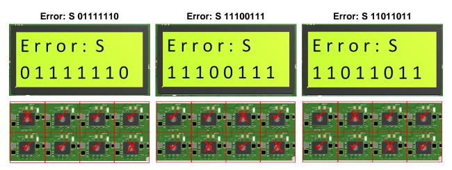
If 8 devices have been placed in the socket and the system still gives this error message, it means that one of the devices was incorrectly placed in the socket; either the leads are not all properly touching or it was place in upside-down. If you wish to replace the IC in the socket, then power down the TIDA-01373 with the ON/OFF switch by switching it to 'OFF' and start back at Section 4.3.2.1.
