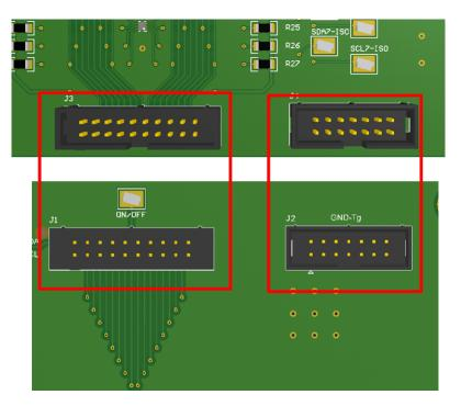
Figure 47. Ribbon Wire Headers on Both Boards
