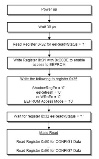
Figure 9. DRV10983-Q1 and DRV10987 Mass Read Protocol Using I<sup>2</sup>C
