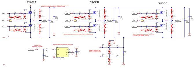
Figure 6-7. Power stage and MOSFETs schematic
