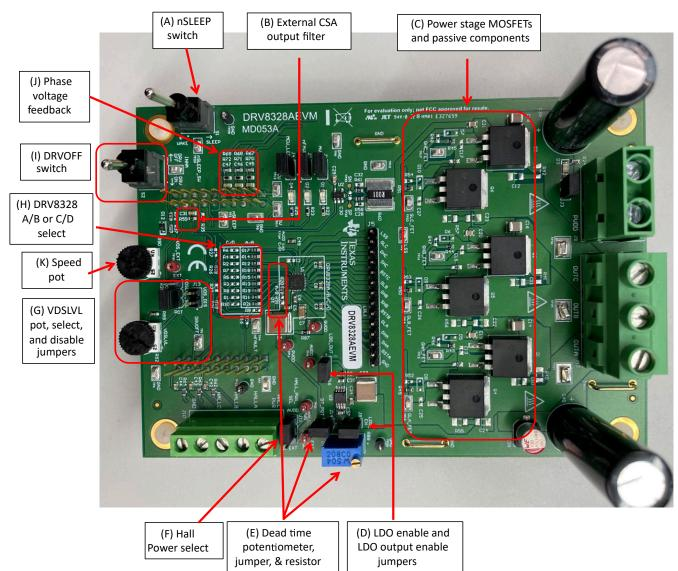
Figure 3-6. User-adjustable jumpers, resistors, and switches on DRV8328AEVM
