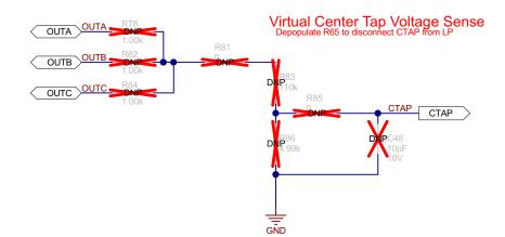
Figure 6-11. Voltage Sense and Protection schematic
