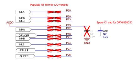
Figure 6-2. DRV8328C/D variant select schematic
