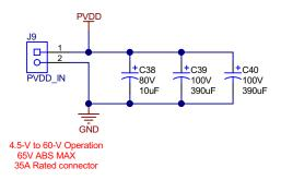
Figure 6-8. Main supply input schematic
