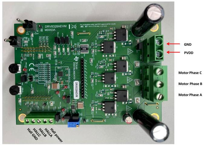
Figure 3-2. Connections from motor to DRV8328AEVM
