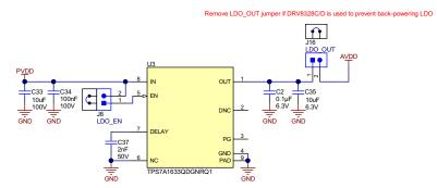
Figure 6-6. External 3.3V LDO schematic
