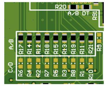
Figure 3-7. Resistors to populate for DRV8328A/B device
