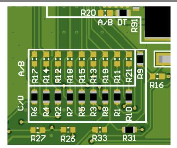
Figure 3-8. Resistors to populate for DRV8328C/D device
