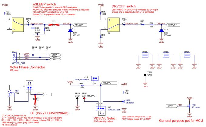
Figure 6-10. Connectors, Selectors, and Analog Control Interface schematic
