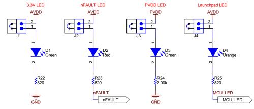
Figure 6-3. Status LEDs schematic
