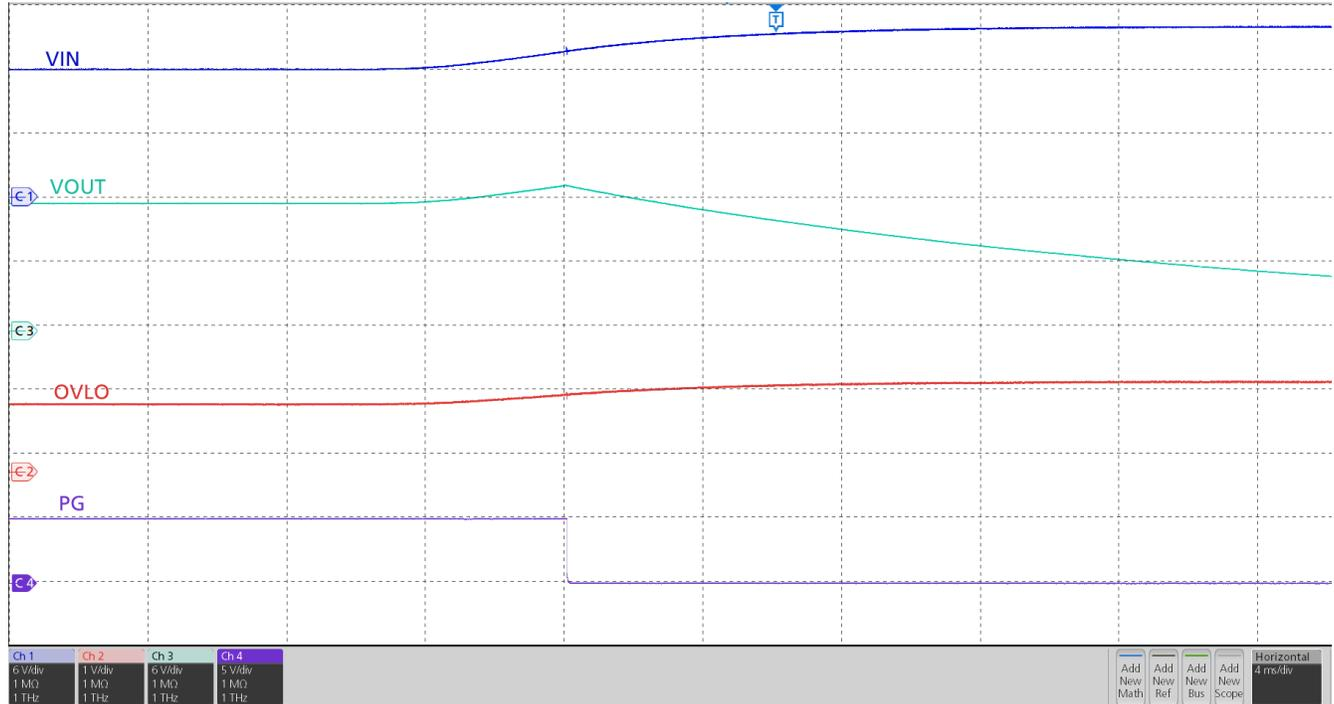
**Figure 5-3. Overvoltage Protection Response of the TPS22811 Device**
