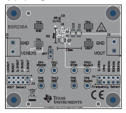
Figure 6-1. PCB Top 2-D (TPSM33625EVM)
