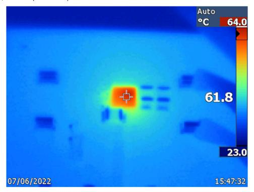
Figure 5-7. IR Top Case Measurement
