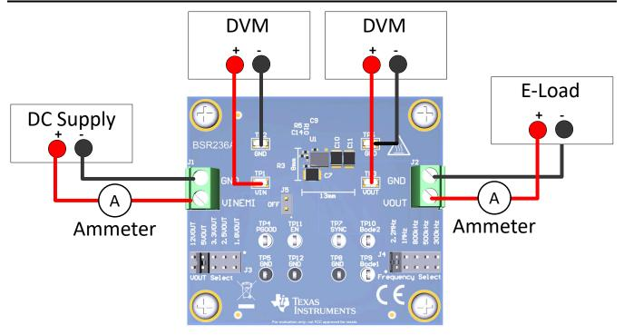
Figure 3-1. Test Setup Diagram
