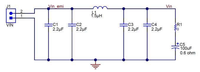
Figure 4-1. Schematic-Compliance Testing Filter
