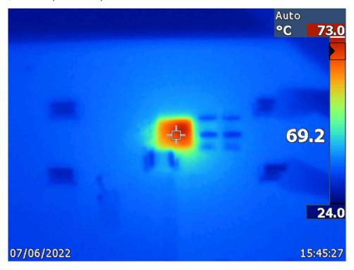
Figure 5-8. IR Top Case Measurement
