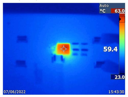
Figure 5-5. IR Top Case Measurement
