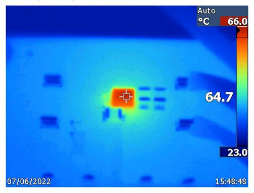
Figure 5-6. IR Top Case Measurement
