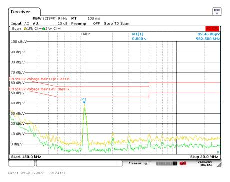
Figure 5-1. CISPR32 Conducted Scan
