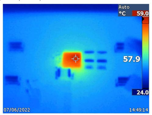
Figure 5-4. IR Top Case Measurement
