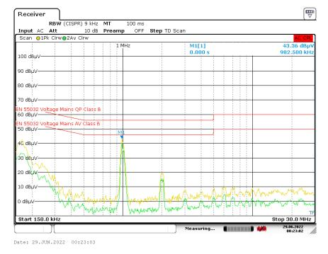
Figure 5-2. CISPR32 Conducted Scan
