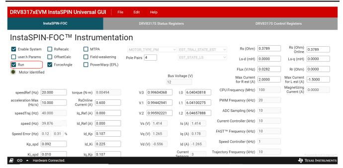
Figure 6-2. C2000 InstaSPIN Universal GUI Running motor identification
