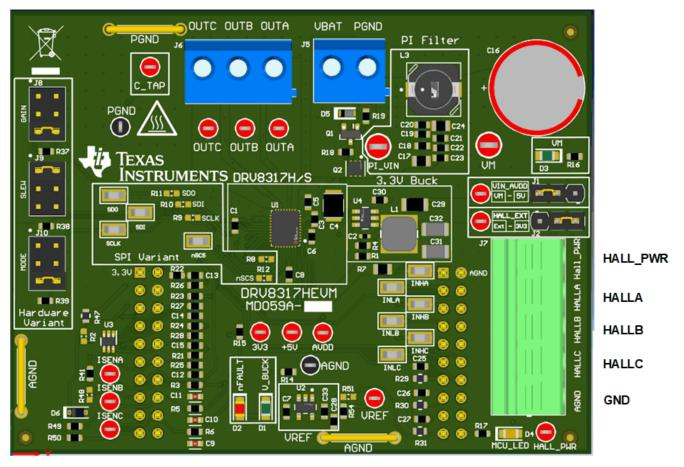
Figure 4-2. Connections from motor to DRV8317HEVM
