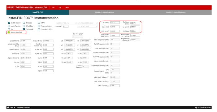
Figure 6-3. Motor identification complete using the DRV8317HEVM InstaSPIN GUI
