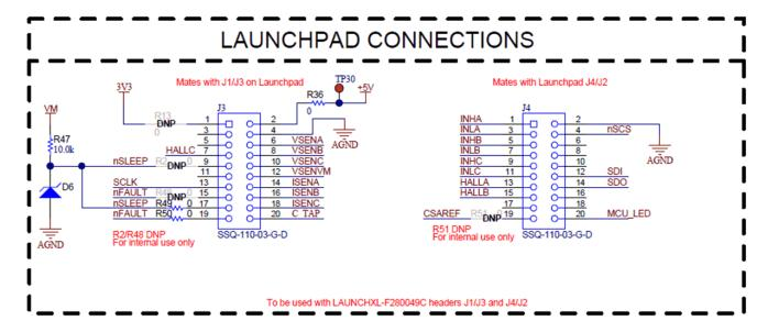
Figure 7-4. LaunchPad Connections schematic
