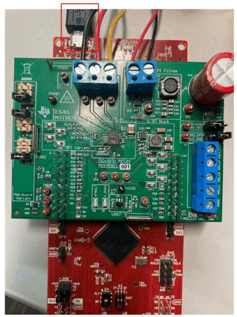
Figure 4-3. DRV8317HEVM on headers J1/J3 and J2/J4 of LaunchPad and Micro-USB plugged into LaunchPad
