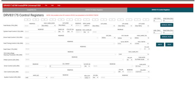
Figure 6-5. DRV8317HEVM InstaSPIN GUI SPI Control Registers
