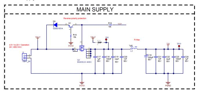
Figure 7-1. Main Supply schematic
