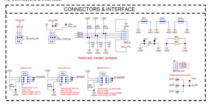
Figure 7-5. Connectors & Interface schematic
