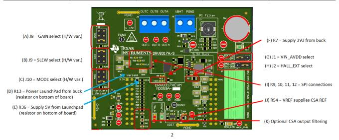
Figure 4-5. User-selectable jumpers and DNP components on DRV8317HEVM
