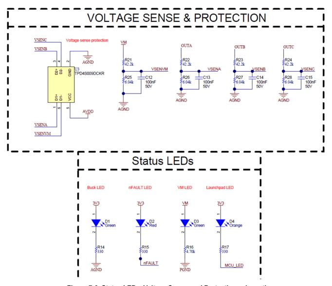
Figure 7-6. Status LEDs, Voltage Sense, and Protection schematic
