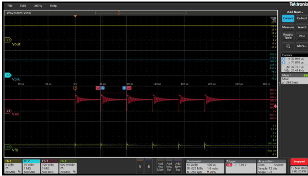
Figure 3-34. 230Vac/0.4W (25kHz Burst Frequency/ Vfb - 0.27V)
