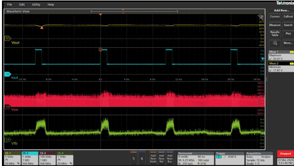
Figure 3-60. VIN=90Vac (2.25x Rated Current for 1ms, 0.9x Rated Current for 9ms)
