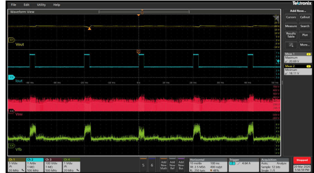
Figure 3-61. VIN=90Vac (2x Rated Current for 2ms, 0.9x Rated Current for 18ms)
