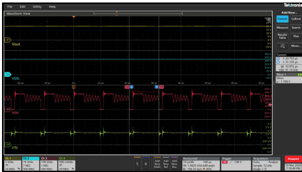
Figure 3-38. 230Vac/40W (91kHz 6 th Valley Switching/ Vfb - 1.71V)
