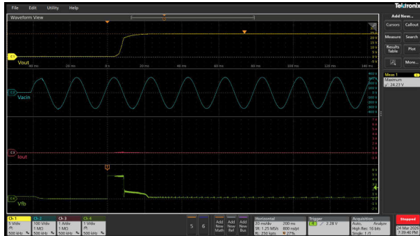
Figure 3-64. Startup Response at 24V and 0A (Overshoot = 230mV)
