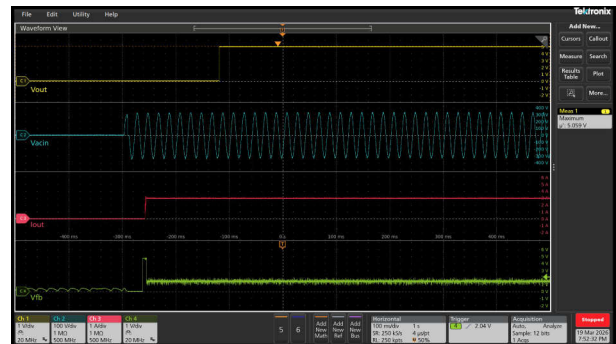
Figure 3-69. Startup Response at 5V and 3A (Overshoot = 59mV)
