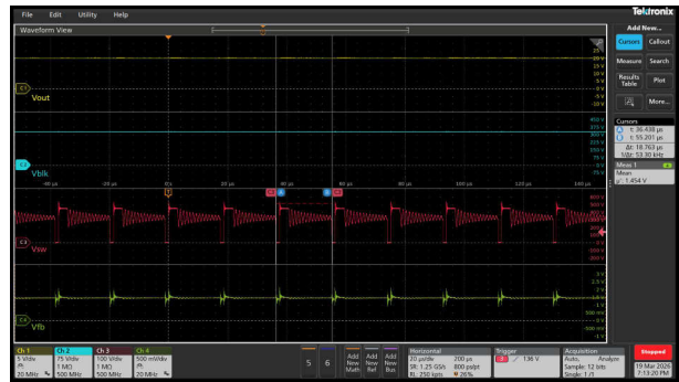
Figure 3-37. 230Vac/16W (53kHz Frequency-Foldback/ Vfb - 1.45V)
