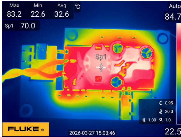
Figure 3-70. Top Side at 90Vac-to-24V/2.71A
