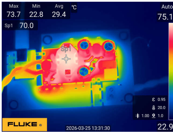
Figure 3-82. Top Side at 230Vac-to-20V/3.25A
