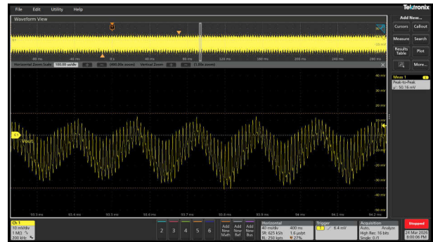
Figure 3-41. Typical Ripple Voltage of V_{OUT} = 24V at Full Load (50mVpp)
