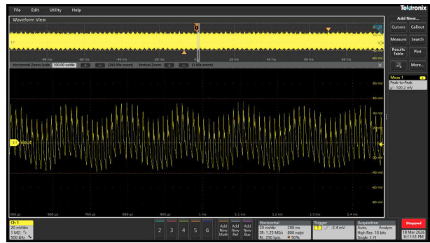
Figure 3-49. Typical Ripple Voltage of V_{OUT} = 9V at Full Load (100mVpp)
