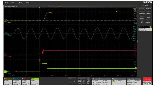
Figure 3-65. Startup Response at 24V and 2.71A (Overshoot = 270mV)
