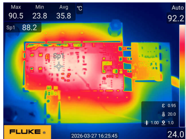
Figure 3-75. Bottom Side at 230Vac-to-24V/2.71A
