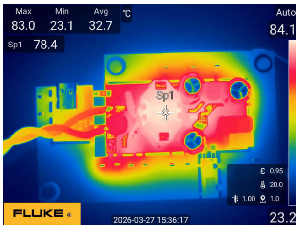
Figure 3-74. Top Side at 230Vac-to-24V/2.71A
