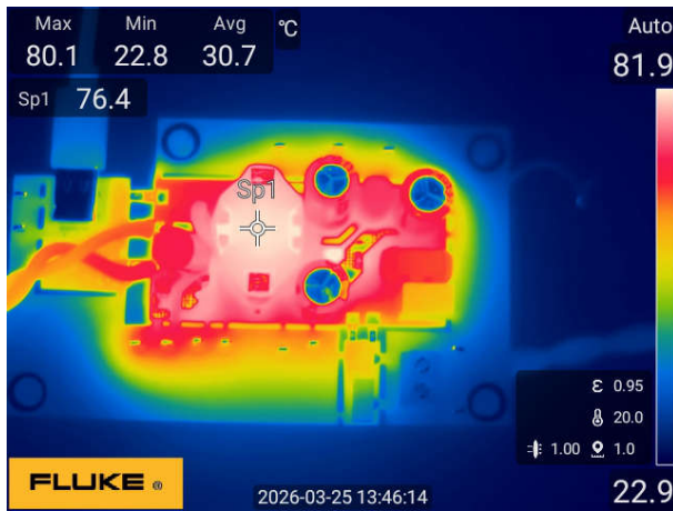
Figure 3-84. Top Side at 264Vac-to-20V/3.25A
