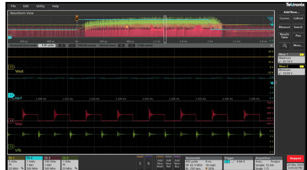
Figure 3-63. VIN=90Vac (2x Rated Current for 2ms, 0.9x Rated Current for 18ms) - Zoomed
