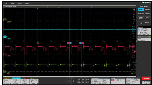
Figure 3-39. 230Vac/65W (115kHz 3 rd Valley Switching/Vfb - 1.93V)
