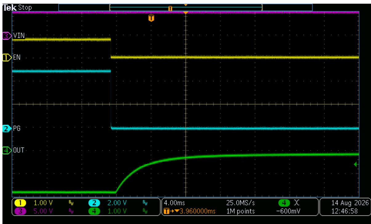
Figure 3-7. Power Good De-assert - EN Independently Driven LOW
