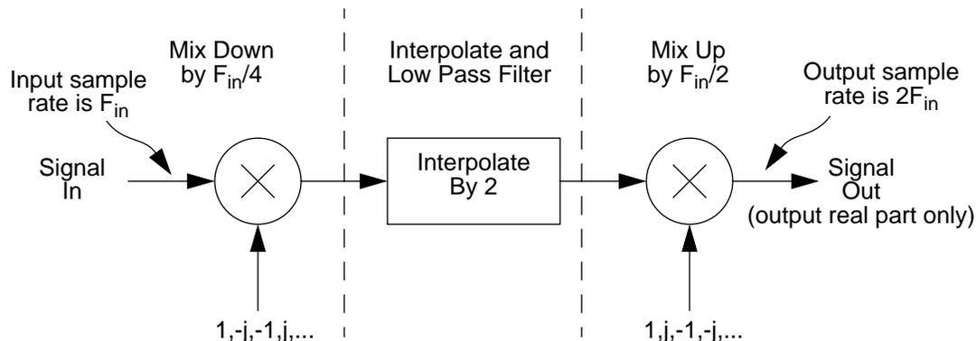
Figure 1. Up-conversion and Interpolation
