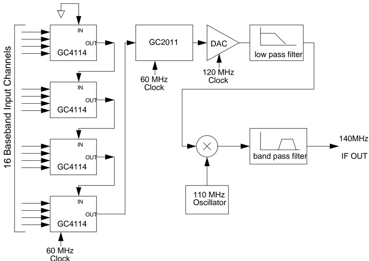
Figure 4. Multi-Carrier Transmit Module Example
