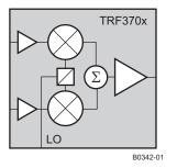
Figure 1. TRF370x Functional Block Diagram
