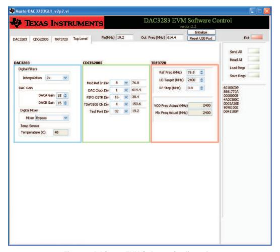
Figure 4. DAC3283 EVM Software Configuration
