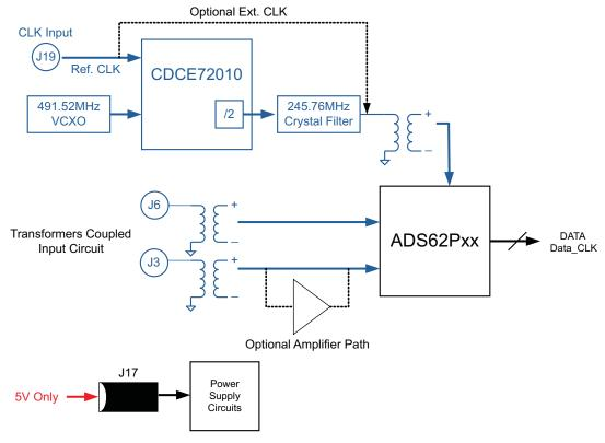
Figure 3. ADS62P49 EVM Block Diagram
