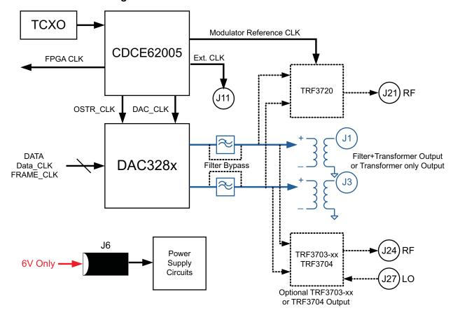
Figure 2. DAC3283 EVM Block Diagram
