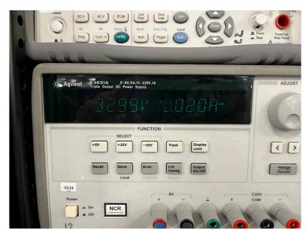
Figure 8-5. IR Encoder Current Consumption
