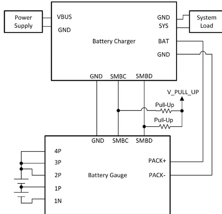
Smart battery system with no host needed
