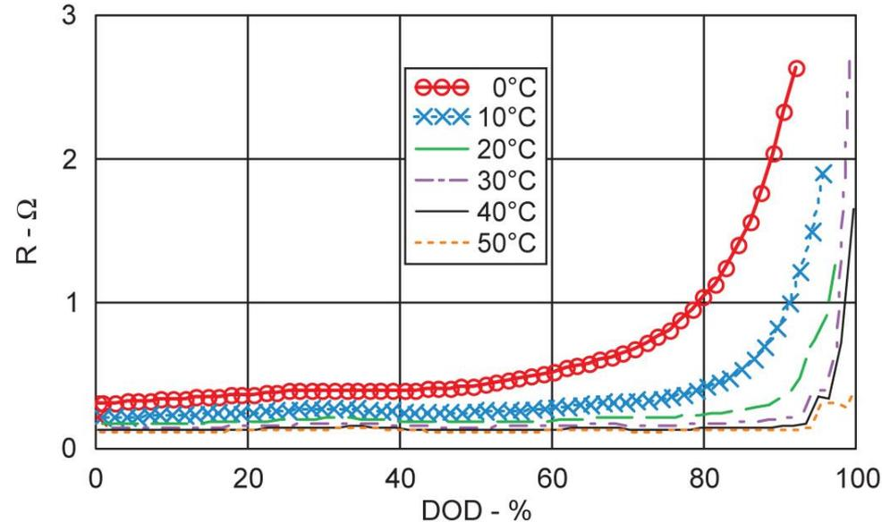
Internal resistance of battery at varying temperatures
