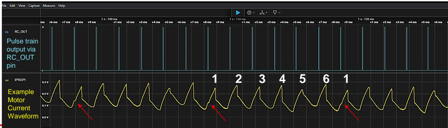
Red arrows indicate repeatability of ripple current waveform. Above scopeshot shows 6 ripples per revolution.
