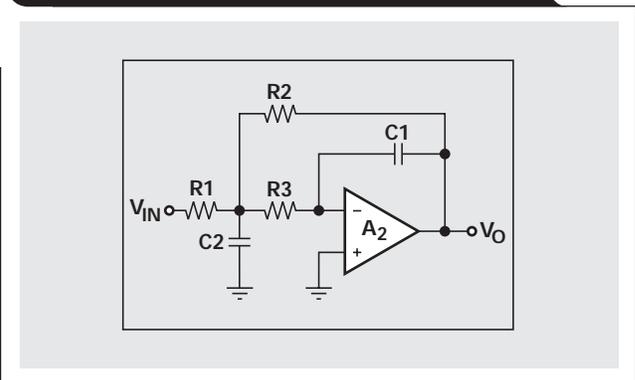
Figure 4. Sallen-Key complex pole-pair section (gain = 1)
