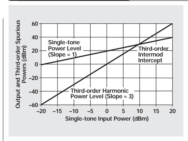
Figure 3. Two-tone, third-order intermodulation intercept amplitudes
