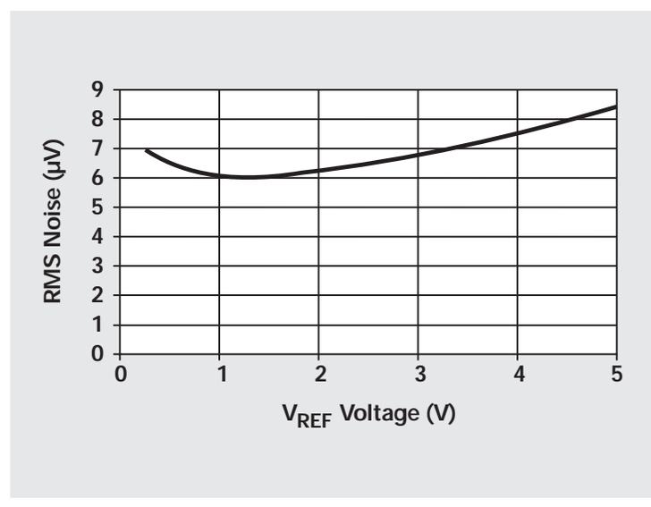
Let's start by looking at the case of a  $V_{REF}$  of 5 V (Figure 3). If the input signal is smaller than the full-scale range of 10 V (-5 V to +5 V), then it would be more useful to plot the noise versus the signal full-scale value. For example, a noise of 5 ppm with a 5-V full-scale is 10 ppm if the full-scale range is only 2.5 V. It is the magnitude of the noise relative to the signal amplitude that holds our main interest.
