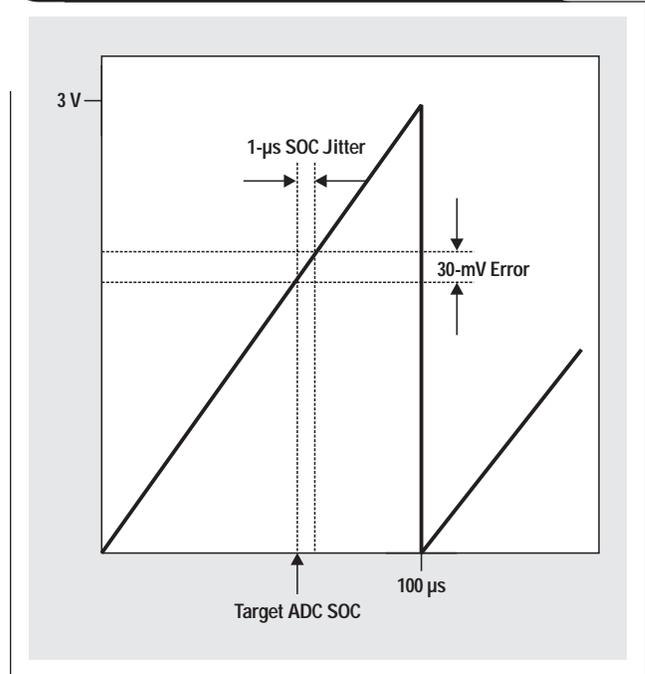
timer clock—all interrupt and latency uncertainty associated with software-driven SOC is removed completely from the system. The ADC10 SOC will be triggered with perfect timing, using the CCRx hardware asynchronously and regardless of other CPU, software, or system activity.
