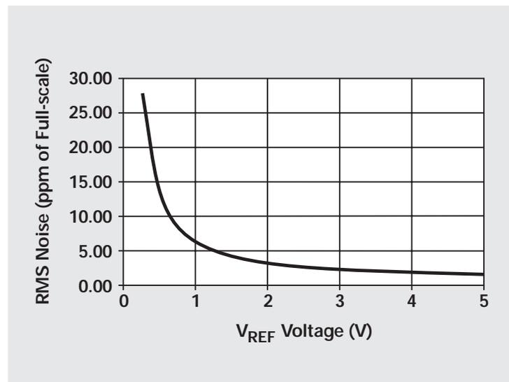
Figure 2. ADS1253 RMS noise vs.  $V_{REF}$  as  $\mu\text{V}$
