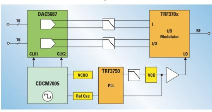
The CDCM7005 is a highperformance, low-jitter clock solution that synchronizes an onboard voltagecontrolled crystal oscillator (VCXO) to an external reference clock. Once the proper reference frequency and programming are applied, the CDCM7005 supplies two clock sources to the DAC and an additional two outputs for external equipment.
