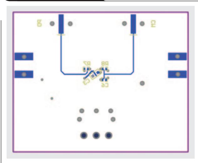
**Adapting the THS4509 test circuit to an IF ADS5424 interface**
