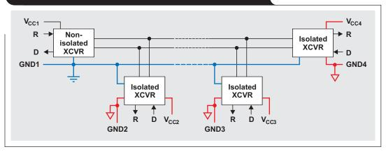
While Figure 8 shows the detailed connection of two remote transceiver nodes, Figure 9 shows an example of an isolated data-transmission system using multiple transceivers. Here all but one transceiver connect to the bus via isolation. The non-isolated transceiver on the left provides the single-ground reference for the entire bus.
