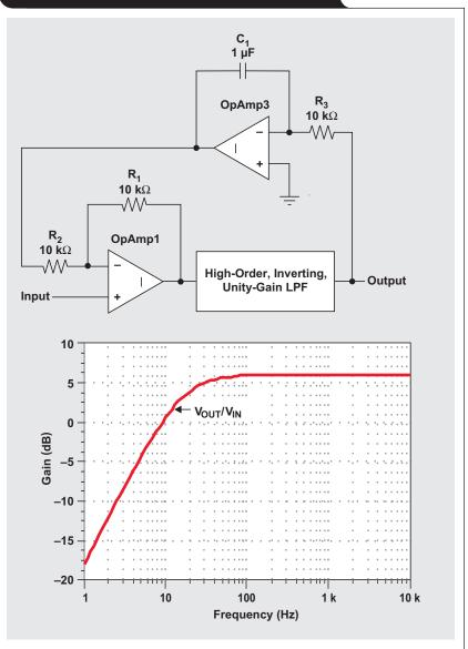
$$f = \frac{\frac{R_1}{R_2}G_{LPF}}{2\pi R_3 C_1}.$$
