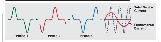
While the third and fifth harmonics of the fundamental 60-Hz line frequency make up the lion's share of the harmonic content, the vector sum of all frequency components (including the 60-Hz fundamental) can reach peak values that exceed the amplitude of the fundamental phase current by more than 100%.
