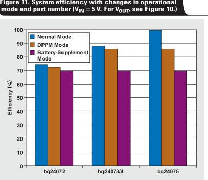
Figure 11. System efficiency with changes in operational
