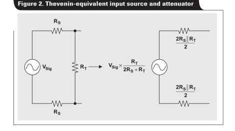
For analysis, it is convenient to assume that the FDA is an ideal amplifier with no offset and has infinite gain. The first step in analyzing the circuit in Figure 1 is to simplify it by using only its attenuator portion and the Thevenin equivalent of the input source. This is shown in Figure 2. With the circuit in this form, it is easier to see that its overall gain can be calculated by the formula
