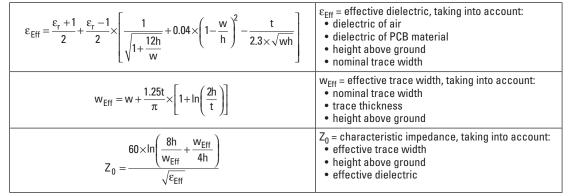
\*Keep all dimensions in inches, mils (1 inch = 1000 mils), or millimeters (1 inch = 25.4 mm).
