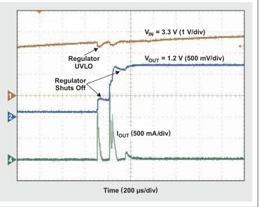
the inrush current of linear regulators designed for fast start-up, like the Texas Instruments (TI) TPS734xx/5xx, which have a high power-supply ripple rejection (PSRR), low noise, and an ultralow  $I_q$ . Figure 2 shows how adding a FET and some passive circuitry to the TPS73525 provides greater control over the inrush current.  $I_{IN}$  is measured between the regulator input pin and the input capacitor because both the capacitor and the input power supply will supply the inrush current.
