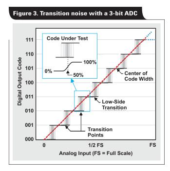
Equation 1 describes the typical transfer function of the ideal (error-free) ADC:
