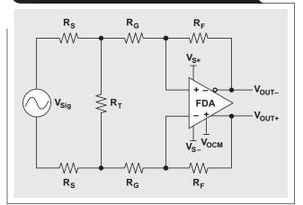
circuit is that the gain resistors can no longer be chosen simply to provide the attenuation. Two approaches are identified in this article; one implements an input attenuator with resistor values chosen to provide a noise gain of 2, and the other implements the attenuator using the gainsetting resistors with added components to get a noise gain of 2.
