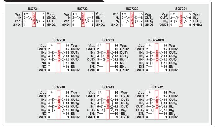
from 3.3 V to 5 V for both supplies,  $V_{\rm CC1}$  and  $V_{\rm CC2},$  and allows any combination of these values.
