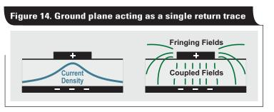
while their electric fields tightly couple. The TEM waves of the two conductors, now being robbed of their magnetic fields, cannot radiate into the environment. Only the far smaller fringing fields might be able to couple outside, thus yielding significantly lower EMI.
