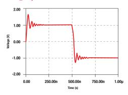
Step response of amplifier with limited capacitive load drive: non-ideal behavior – ringing effect, slow recovery
