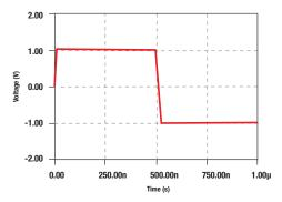
Step response of amplifier with large capacitive load drive: smooth transient response
