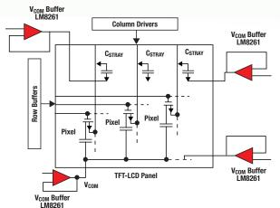
Displays with larger screens and those that are touch-based often require more than one  $V_{\text{COM}}$  buffer.
