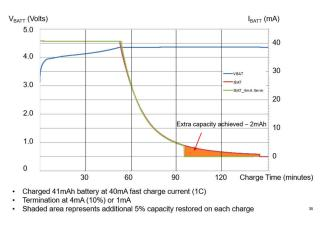
Figure 2. Extra capacity from a lower I<sub>TERM</sub>.
