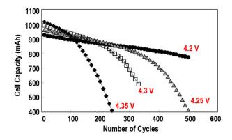
Figure 3. Li-ion cell capacity vs. number of recharge cycles.
