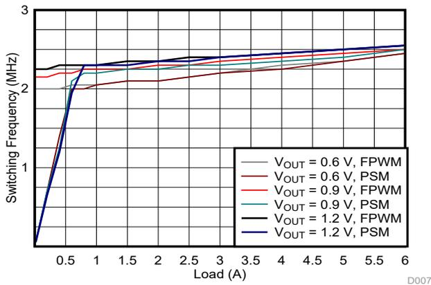
**Figure 4.** Switching frequency variation of the TPS62869 with DCS-Control.
