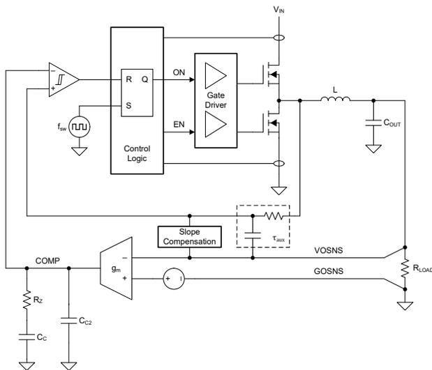
**Figure 2.** Block diagram of the **TPS62873**'s fixed-frequency DCS-Control topology with the oscillator, differential remote sensing, transconductance amplifier and hysteresis comparator.
