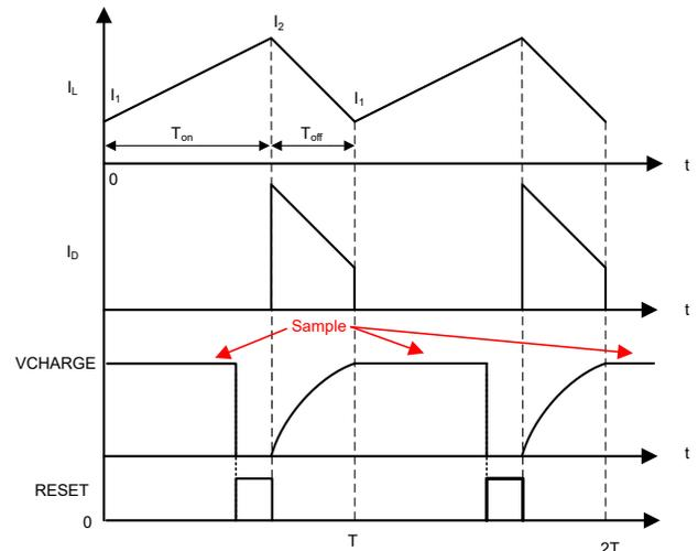
**Figure 5.** Typical signal waveforms for charge-mode control.
