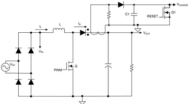
**Figure 4.** Using a CT to obtain an electric charge.
