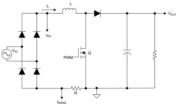
**Figure 1.** A common current-sensing method for PFC.
