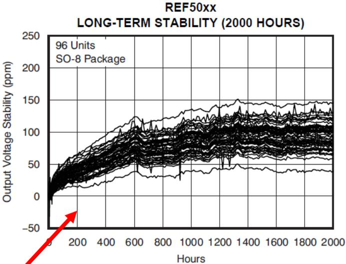
**The initial shift (first few months) makes up the majority of change. Self curing of molding compound.**
