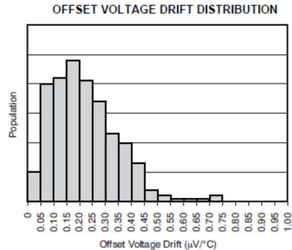
Max LT Vos drift = 2.0 $\mu\text{V}/^\circ\text{C}$
