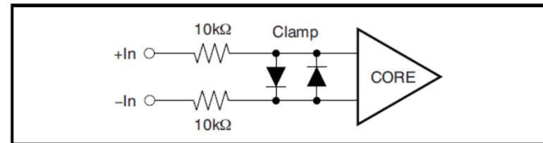
Figure 19. Equivalent Input Circuit
