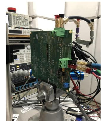
Fig. 3. Photograph of the TPS7H4001-SP mounted on the TPS7H4001EVM-CVAL in front of the heavy-ion beam port exit at the TAMU cyclotron facility.
