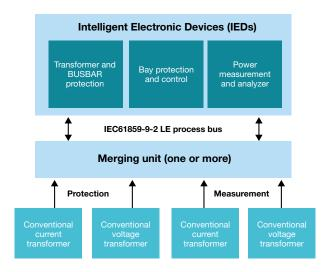
Figure 3. A merging unit with a conventional transformer
