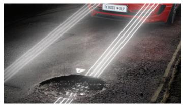
*Figure 6. DLP headlights working with the ADAS camera systems to detect and alert drivers to objects in the road.*
