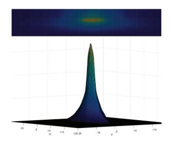
Figure 3. Typical high-beam illumination profile with a high-center peak.
