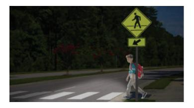
*Figure 7. DLP headlights highlight a child attempting to cross the street while dimming the crosswalk sign to reduce glare.*
