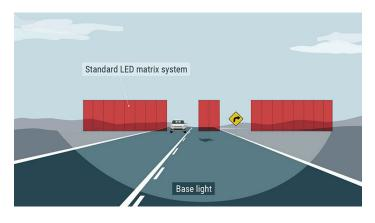
*Figure 2.* Headlight FOV with a background 12-pixel matrix. Each pixel is illustrated with the red segment in the high beam FOV.
