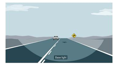
Figure 1. Headlight FOV with only a base light module.
