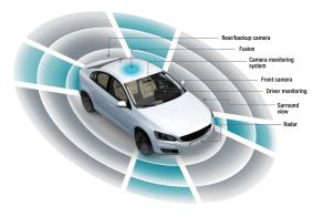
*Figure 3.* Radar sensing for ADAS showing the range of view for multiple cameras and sensors.
