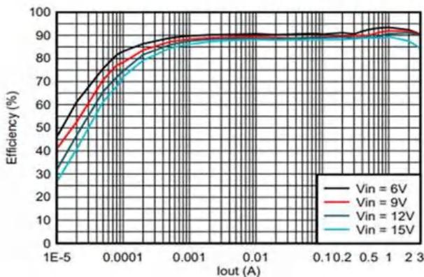
**Figure 6.** Efficiency versus output current (3.3V<sub>OUT</sub> at 2.5MHz, 1 $\mu$ H, automatic PFM or pulse-width modulation).
