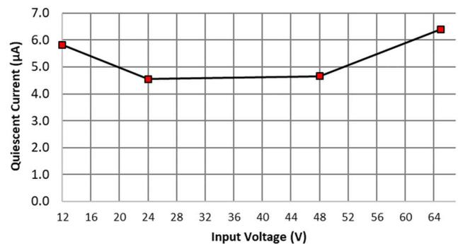
**Figure 5.** The **LMR365R0X** and **TPSM365R15**  $I_Q$  at  $FSW = 1MHz$  and  $V_{OUT} = 3.3V$
