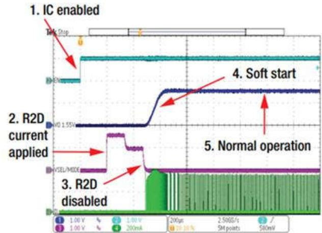
**Figure 4.** The power-supply IC is enabled, followed by R2D circuit operation with two current source levels, soft start and normal operation.
