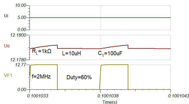
Figure 331. Transient Simulation of a Boost Circuit with High-Frequency, Small Inductance and Light Load
