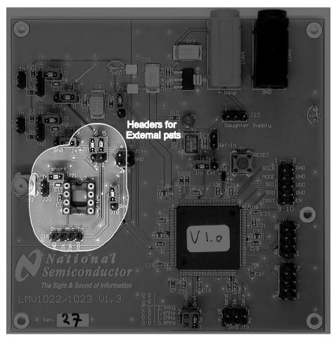
Figure 5. Settings for External Parts Connected to the Demo Board
