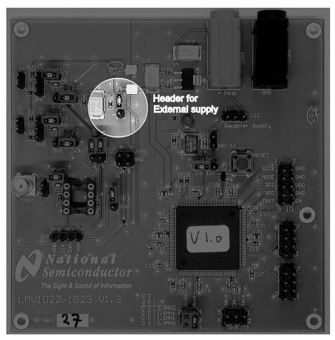
Figure 4. External Controlled Supply Voltage
