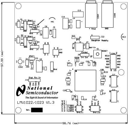
Figure 13. Silk-screen LMV1022 / LMV1023 Demo Board
