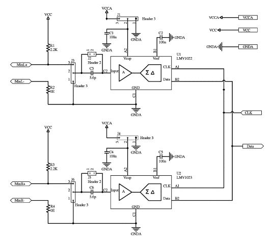
Figure 20. On-board Parts LMV1022 / LMV1023 Demo Board
