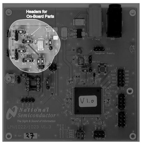
Figure 3. Setting for Testing the On Board LMV1022 and LMV1023
