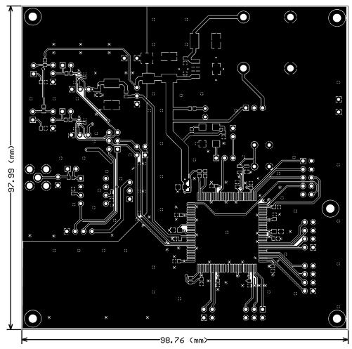
Figure 14. Top Layer LMV1022 / LMV1023 Demo Board
