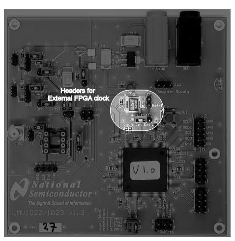
Figure 7. External FPGA Clock
