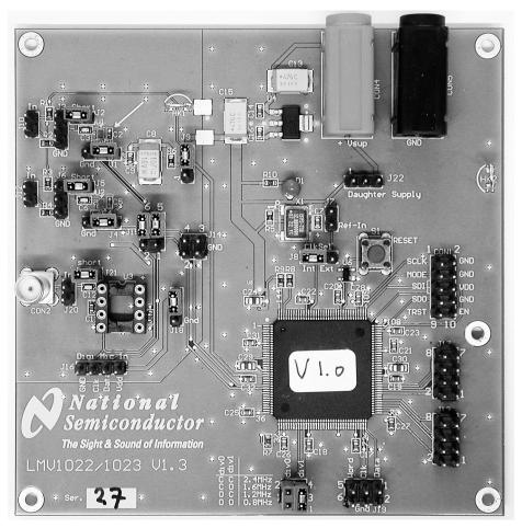
Figure 1. LMV1022 / LMV1023 Digital Output PDM Microphone Amplifier Demo Board
