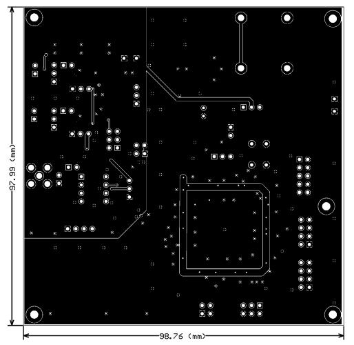
Figure 15. Bottom Layer LMV1022 / LMV1023 Demo Board
