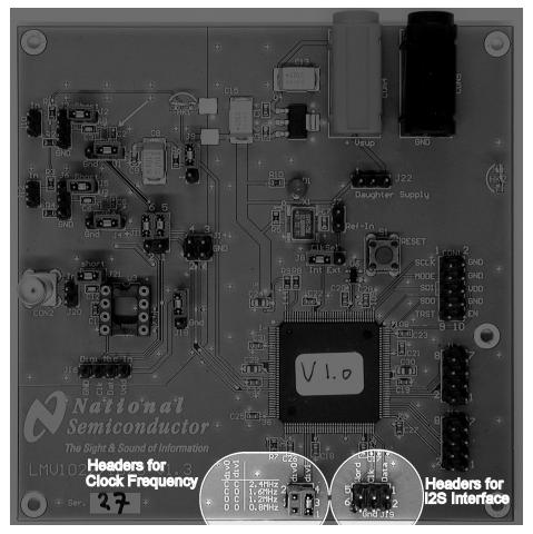
Figure 6. Clock Rate and I2S Interface
