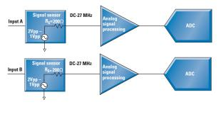
Figure 2. Two signal-path receiver system
