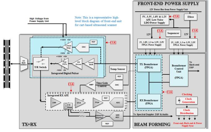
Figure 1-1. Representative Block Diagram (Front-end Unit)
