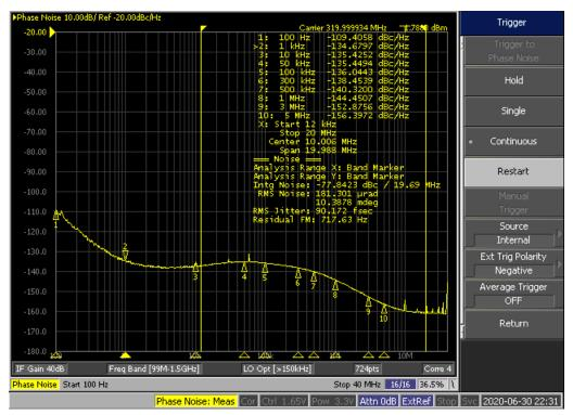
Reference = 320 MHz LVPECL Integrated RMS Jitter (12 kHz-20 MHz) - 90 fs
