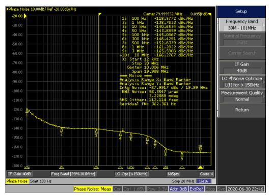
Reference = 320 MHz from LMK61E2 and LMK04832 output = 80 MHz LVPECL Integrated RMS Jitter (12 kHz-20MHz) - 112 fs
