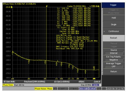
Input = 80 MHz from LMK04832 and output = 80 MHz LVPECL Integrated RMS Jitter (12 kHz-20 MHz) - 132 fs
