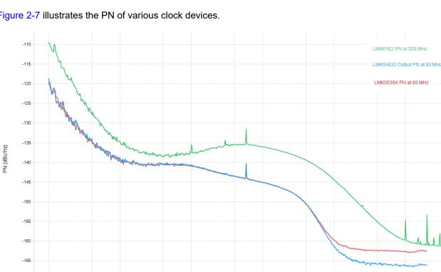
Figure 2-7 illustrates the PN of various clock devices.
