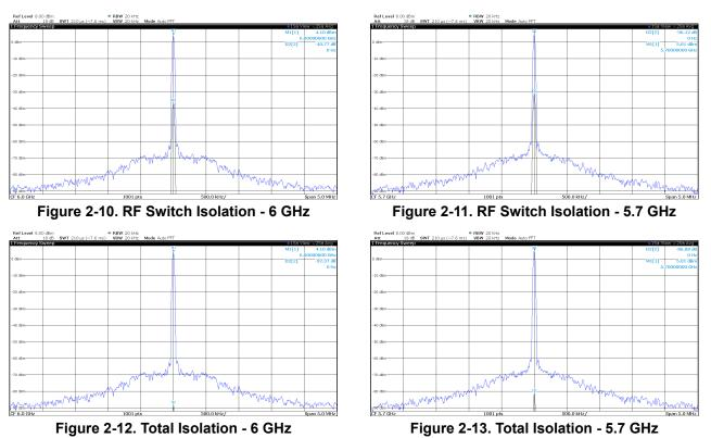
Attenuation from the MUTE pin is approximately 50 dB. RF switch provides another 36 to 40 dB isolation. The total attenuation when the channel is unmuted and switched out is 86 to 90 dB. In other words, when one of the LMX2820 is routed to the output of the RF switch, the user can continue to measure the signal from the other LMX2820 with an isolation of 86 to 90 dB.
