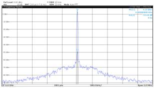
Figure 2-8. MUTE Pin Attenuation - 6 GHz
