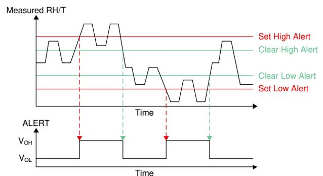
**Figure 1. Graphical Illustration of ALERT Programmable Environmental Thresholds**
