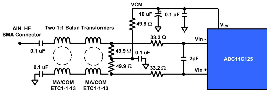
Figure 3. Analog Input Network of ADC11C125HFEB:  $F_{IN} > 150$  MHz
