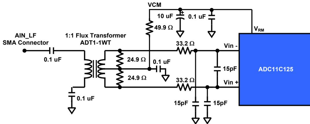
Figure 2. Analog Input Network of ADC11C125LFEB:  $F_{IN} < 150$  MHz
