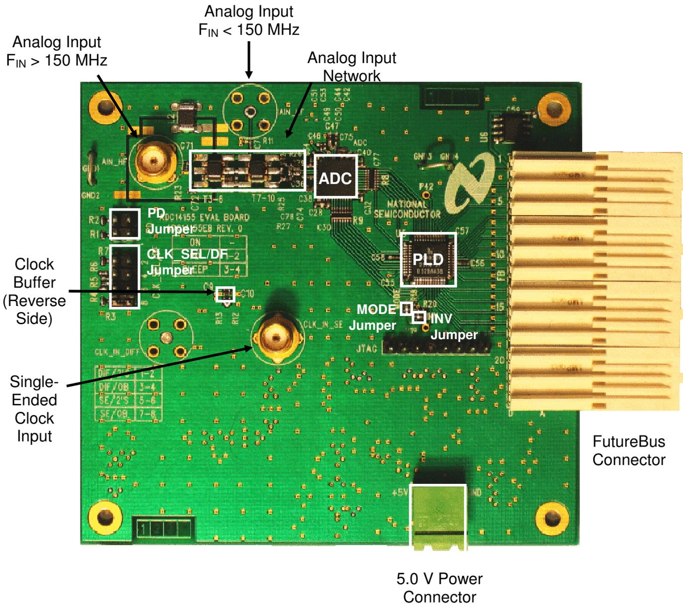
Figure 1. ADC11C125 Evaluation Board Connector and Jumper Locations
