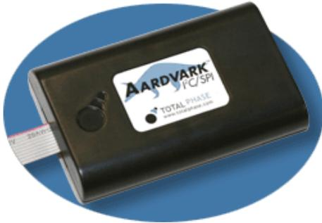
Figure 6. Aardvark I2C/SPI Host Adapter
