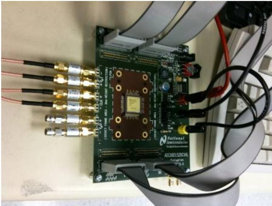
Figure 2. ADC08D1520CVAl Evaluation Board Setup
