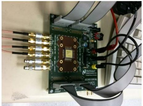
Figure 2. ADC08D1520CVAL Evaluation Board Setup
