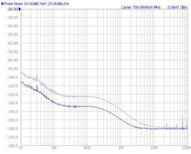
Figure 4-3. 3200MHz Divide by 2 Mode Signal Analyzer Plot
