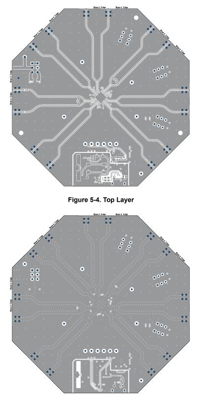
Figure 5-5. Layer 2 (RF GND)
