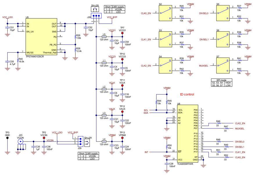
Figure 5-1. Power Supply, IO Control, Switches
