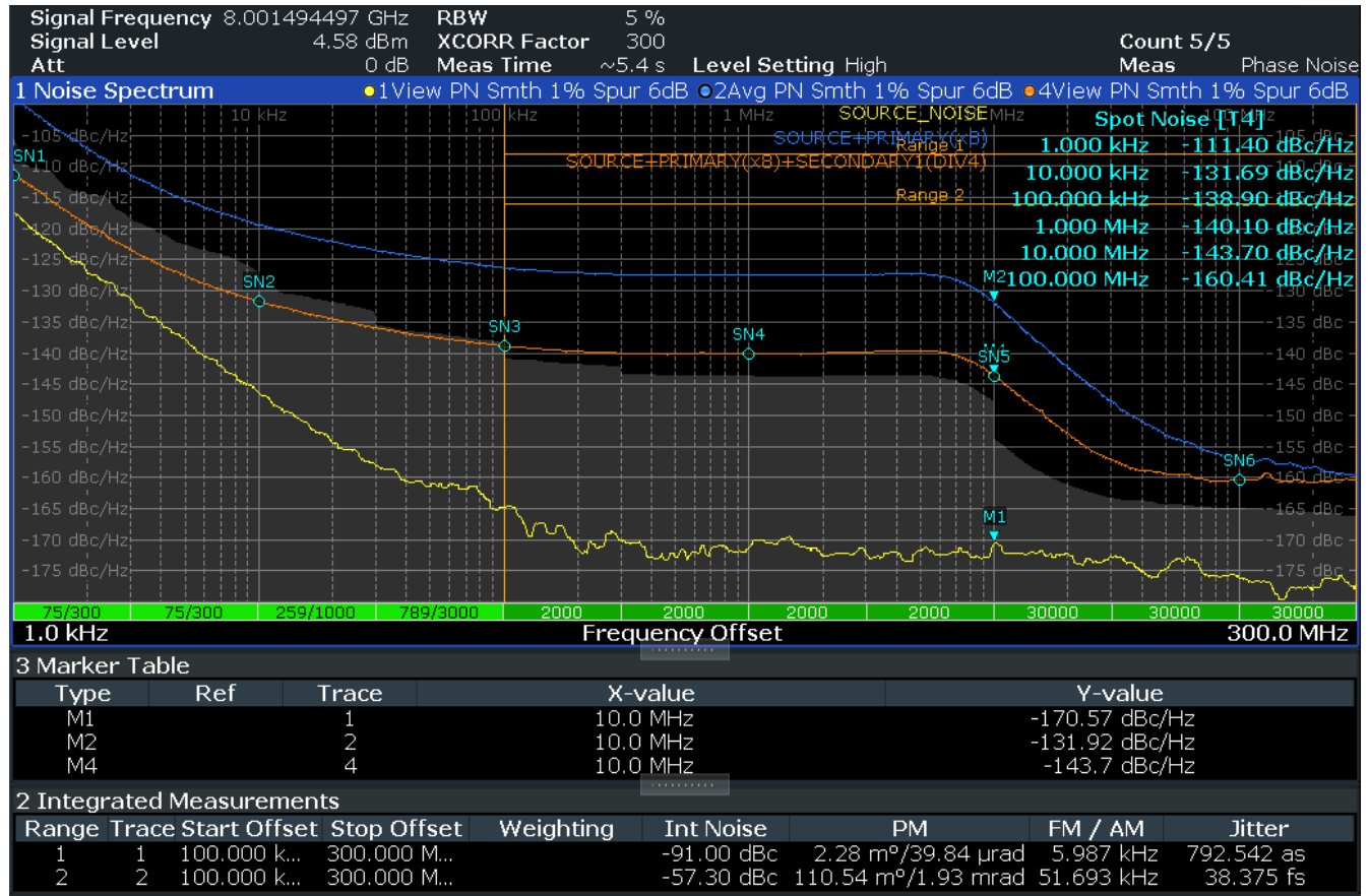
Figure 4-6. Phase Noise Plots for Multiplier Mode ( \times 8 ), 1GHz Reference, and ( \div 4 ) Divider Mode
