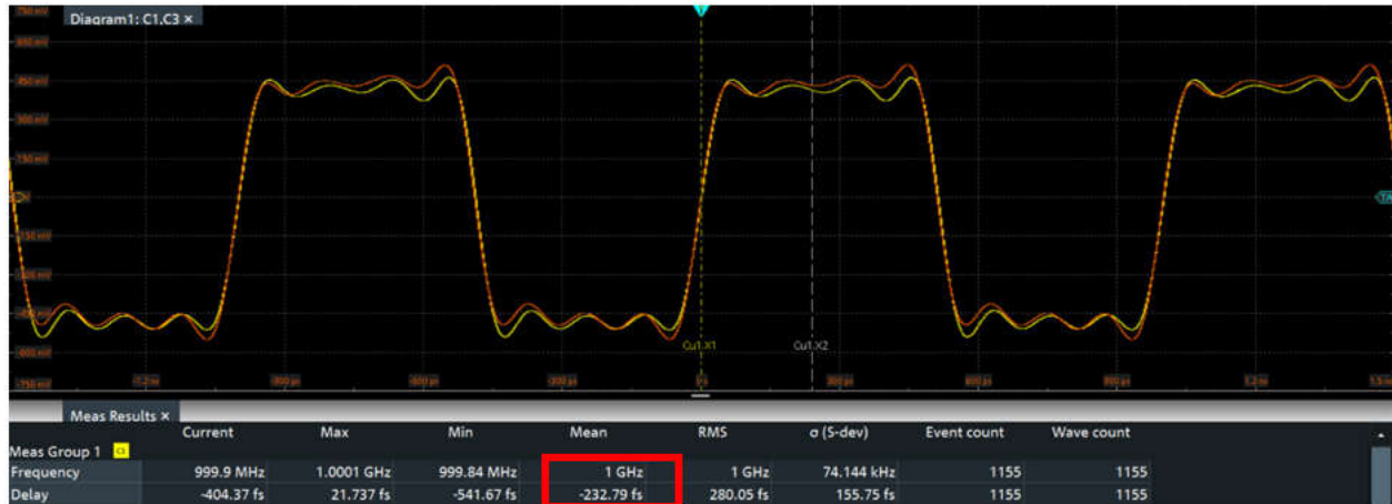
Figure 4-14. Channel to Channel Skew After Adjusting the Output Delay of the Clock Path
