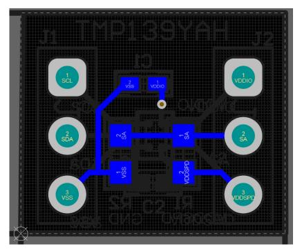
Figure 3-2. TMP139 Breakout Board Bottom Layer
