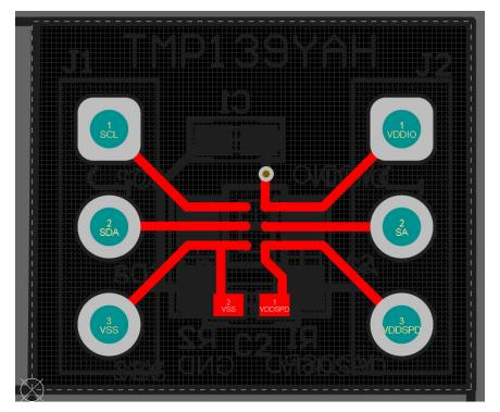
Figure 3-1. TMP139 Breakout Board Top Layer
