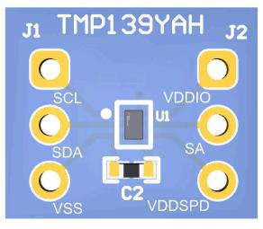
Figure 1-1. Top of TMP139 Breakout Board
