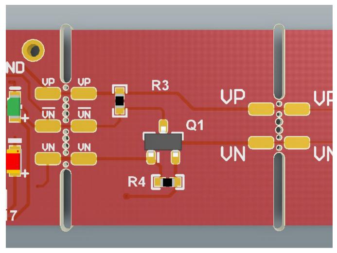
Figure 12. Breakout Slots and Exposed Pads
