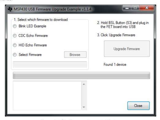
Figure 5. USB Firmware Upgrade Window
