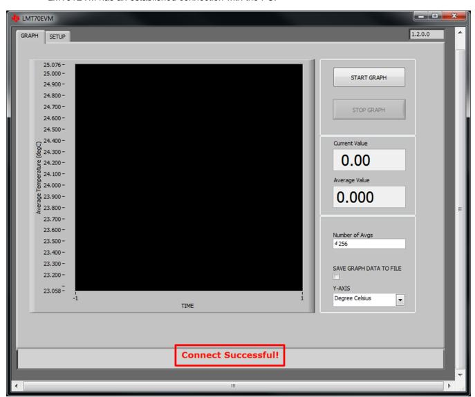
Figure 6. LMT01EVM Successful Connection with PC
