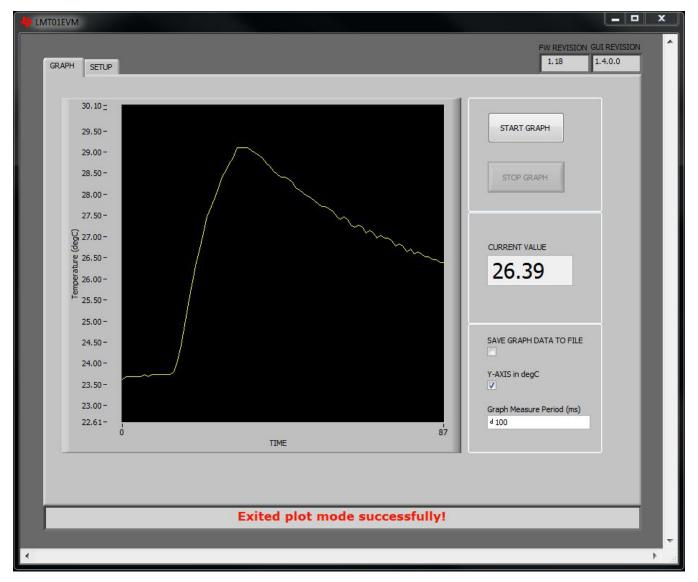
Figure 11. Temperature Change by Pressing Finger on LMT01
