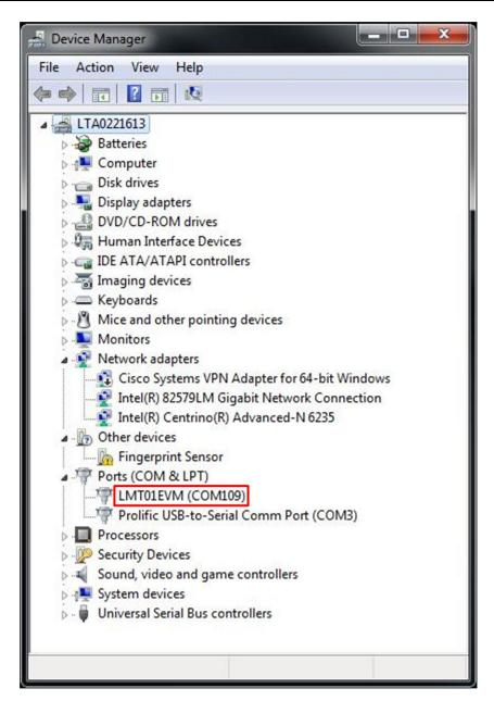
Figure 14. Device Manager with COM Port Name
