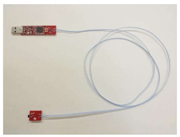
Figure 13. LMT01EVM with LMT01 Device and Microcontroller Connected with Wires
