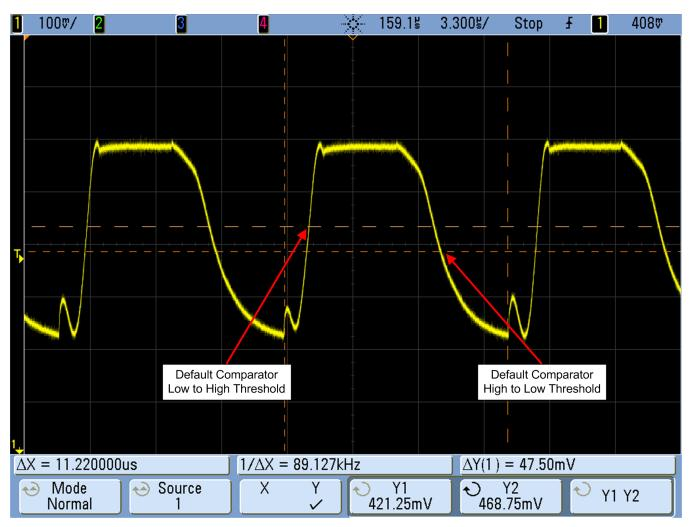
Figure 9. Comparator Threshold
