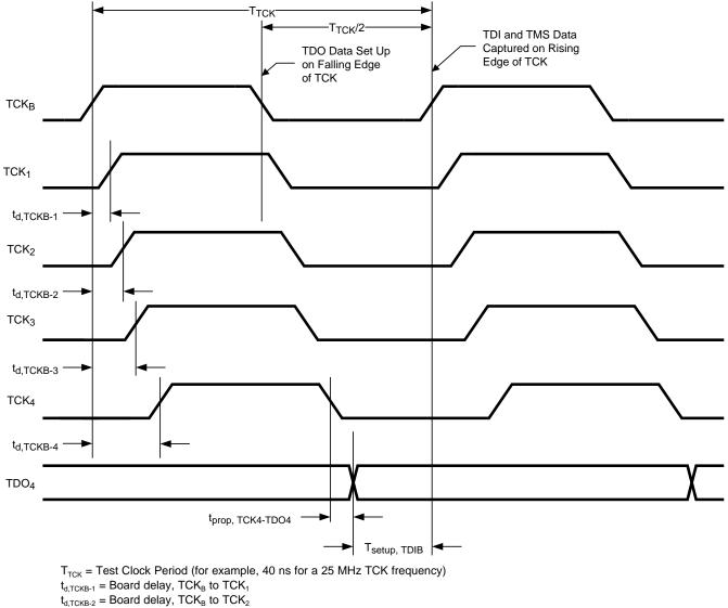
$t_{d,TCKB-3}$  = Board delay, TCK<sub>B</sub> to TCK<sub>3</sub>
