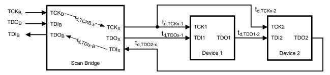
Figure 2. Block Diagram of JTAG Application With the Scan Chain Partitioned Using a Scan Bridge
