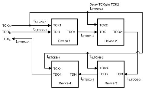
Figure 1. Block Diagram of JTAG Application With a Single TAP
