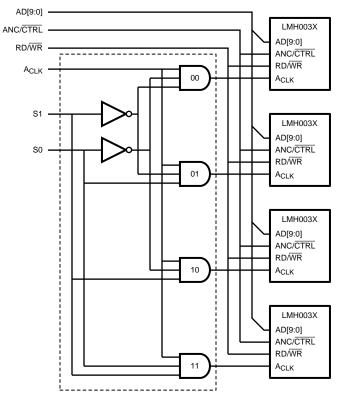
Figure 1. A<sub>CLK</sub> Control Logic
