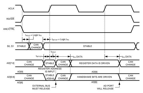
Figure 4. Read Cycle Timing Diagram
