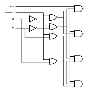
Figure 2. A<sub>CLK</sub> Control Logic with Broadcast Mode
