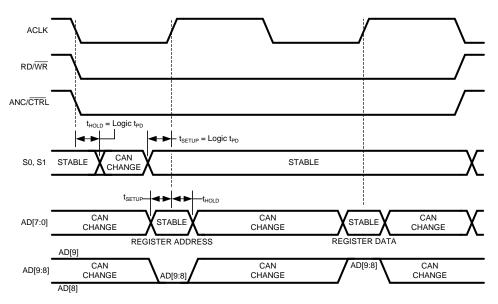
Figure 3. Write Cycle Timing Diagram
